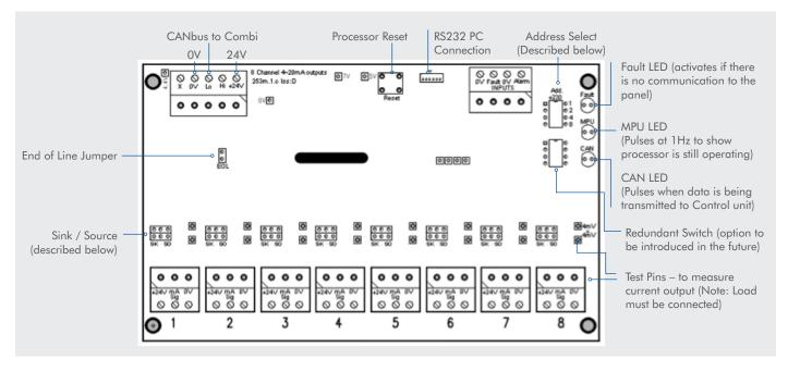
The Combi detects the address being used on this card when connected to the CAN-bus. According to the address, the outputs represent the following:
