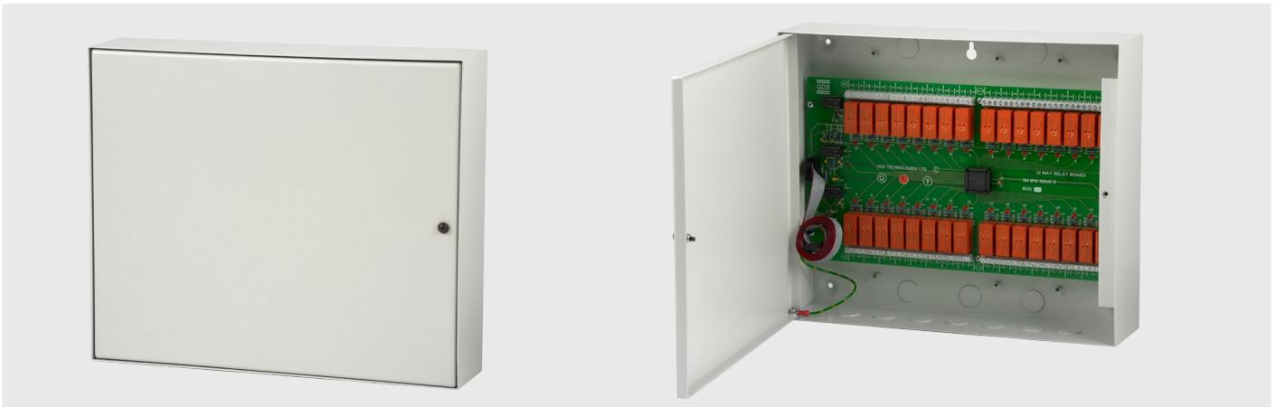
The 32 way relay panel accepts relay data from the combi control unit. It must have a unique address between 128 and 255. This can be selected using the SW1 binary address switch (see example). Ensure that its address does not conflict with another CAN bus device.
